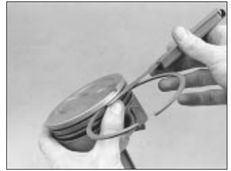
18.10 Check the ring side clearance with a feeler gauge at several points around the groove
