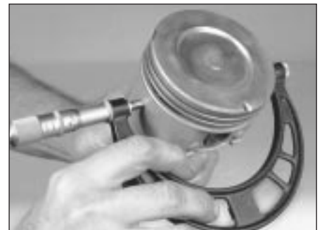
18.11 Measure the piston diameter at a 90-degree angle to the gudgeon pin, at the same height as the gudgeon pin
