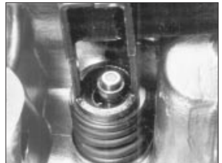
11.6 With the retainer fitted, compress the valve spring and refit the collets as shown
