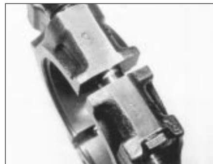
12.4 Mark the big-end bearing caps in order from the front of the engine to the rear (one mark for the front cap, two for the second one and so on)
