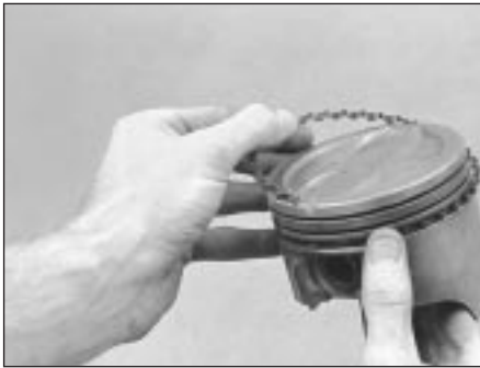
22.9a Refitting the spacer/expander in the oil control ring groove
