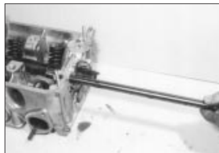
8.13 Removing a rocker arm shaft from the front of the cylinder head - the shaft must be either driven out from the rear of the head with a hardwood dowel or, on models where the rocker shaft is threaded at the front, pulled out from the front with a slide-hammer-type puller
