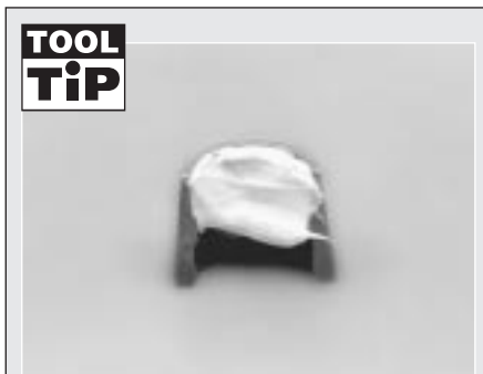
Apply a small dab of grease to each collet to hold it in place, if necessary.
