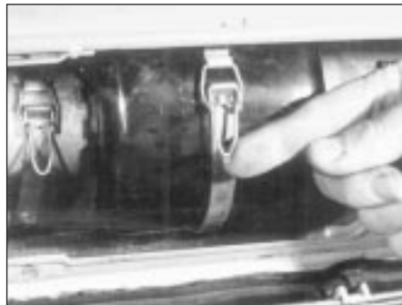
9.5a Unclip the retaining strap to remove the blower housing . . .
