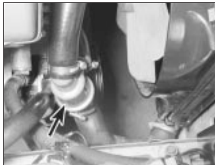
3.8 On the M10 (four-cylinder) engine, the thermostat (arrowed) is connected in-line in the radiator hose
