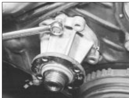
7.18a With the water pump mounting bolts removed, screw two bolts into the special lugs (one top and one bottom) . . .
