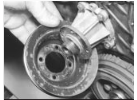
5.29 Removing the water pump pulley (M40 engine)
