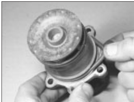
7.23 Fit a new O-ring on the M40 engine water pump
