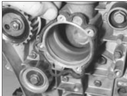
7.24 New outer gasket on the M40 engine water pump
