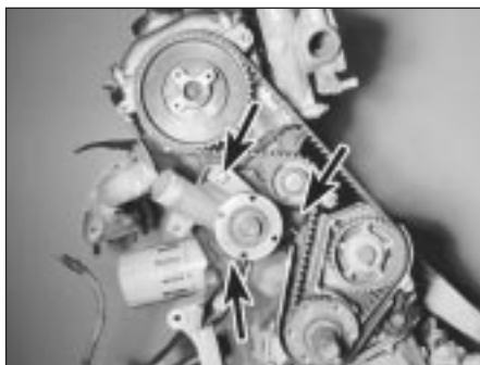
7.12 Water pump bolt locations on the M20 engine
