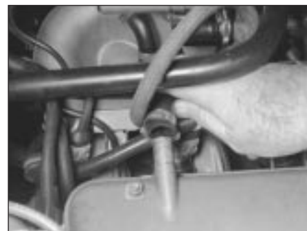
5.2 PCV hose being removed from the valve cover
