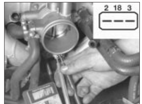
4.28b First check for continuity between terminals 2 and 18 with the throttle closed (later Motronic system shown) . . .
