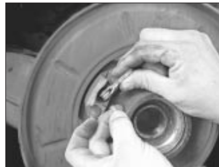
10.4b . . . then remove the pin securing the cable to the inner cam, and remove the inner cam
