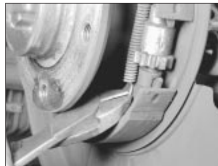
12.7a Remove the lower shoe return spring (diagonal cutting pliers are being used here because they grip the spring well, but care must be taken not to cut or nick the spring)
