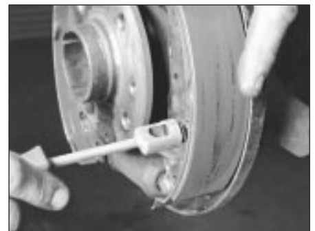
6.6b . . . and the rear shoe hold-down spring
