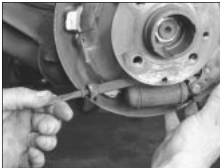
6.8 Remove the automatic adjuster assembly
