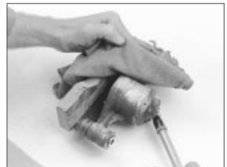
4.5 With the caliper padded to catch the piston, use low pressure compressed air to force the piston out of its bore - make sure your fingers are not between the piston and the caliper
