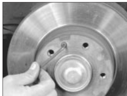
5.6a Remove the disc retaining screw . . .
