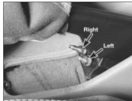
10.1 Peel back the handbrake lever boot and remove the relevant handbrake cable adjusting nut (both arrowed)
