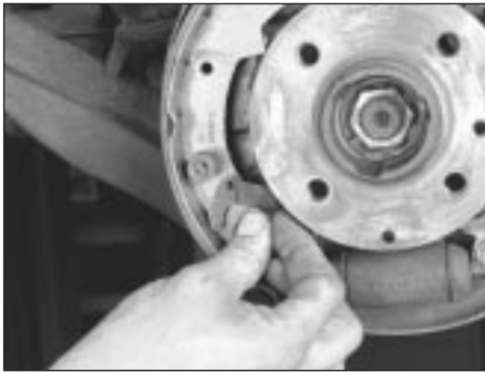
6.13a Refit the automatic adjuster lever first - make sure it's properly engaged with the notch in the front end of the adjuster mechanism . . .
