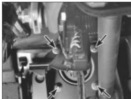
8.10 Remove the four mounting nuts (arrows) and withdraw the servo unit from the engine compartment (left-hand-drive model shown)
