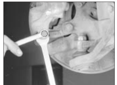
3.5c Hold the guide pins while loosening the caliper mounting bolts (3-Series)
