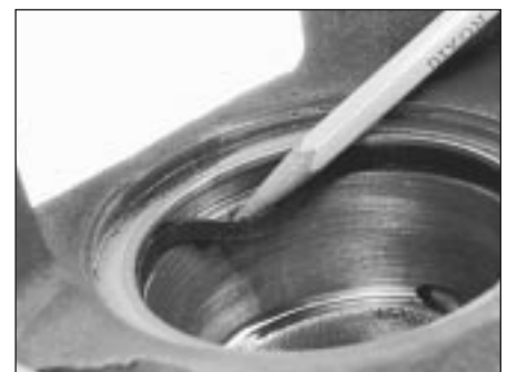
4.7 Remove the piston seal from the caliper bore using a wooden or plastic tool (metal tools may damage the cylinder bore)
