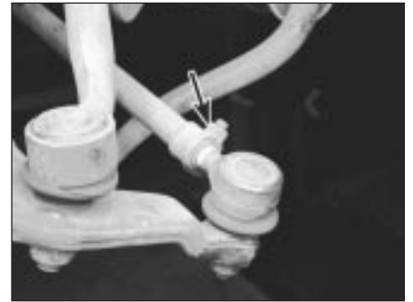
17.6 Measure the length of the track rod and record your measurement, or paint an alignment mark on the threads to ensure the track rod end is refitted in the same position, then loosen the clamp bolt (arrowed)
