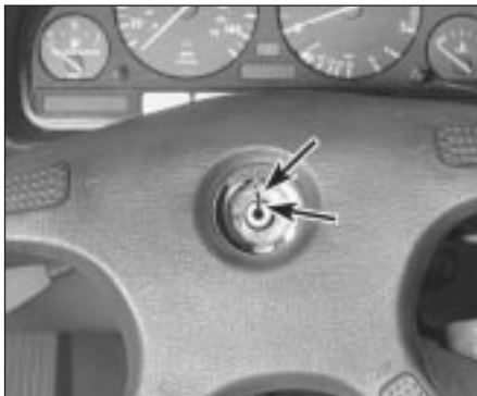
24.3 After removing the steering wheel nut, mark the relationship of the steering wheel to the steering shaft (arrowed) to ensure proper alignment during reassembly
