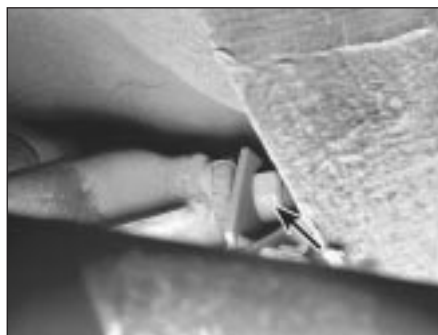
13.6 Nut (arrowed) for the outer pivot bolt
