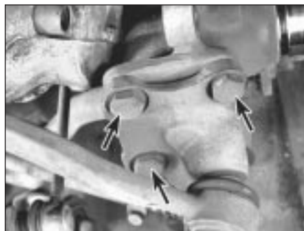
4.5 If you're removing the control arm, remove the three bolts (arrowed) from the steering arm, and separate the strut assembly from the arm
