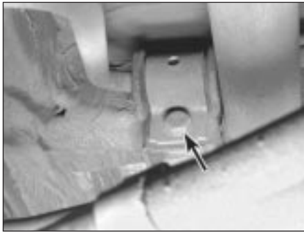
12.2 Rear anti-roll bar bracket bolt (arrowed) (3-Series)
