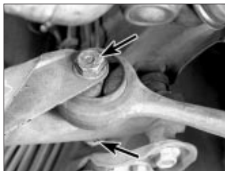
4.6b If you're removing the thrust arm, remove the nut and bolt (arrowed) that secure the rear end of the arm
