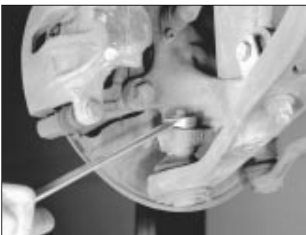
3.13a Remove the self-locking nut from the balljoint stud which attaches the outer end of the control arm to the steering knuckle. If you don't have a balljoint separator tool . . .
