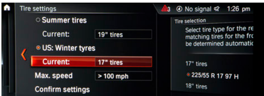
Adjustment of the tire sizes to be set on new wheels in the Central Information Display using the example of the G30
