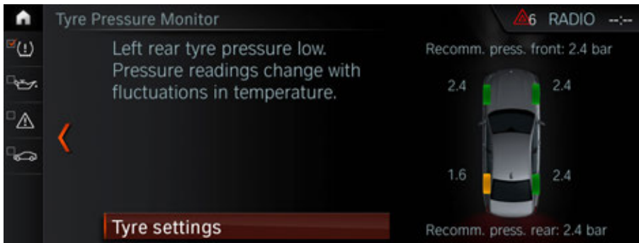
Warning of tire pressure loss using the example of the G30
