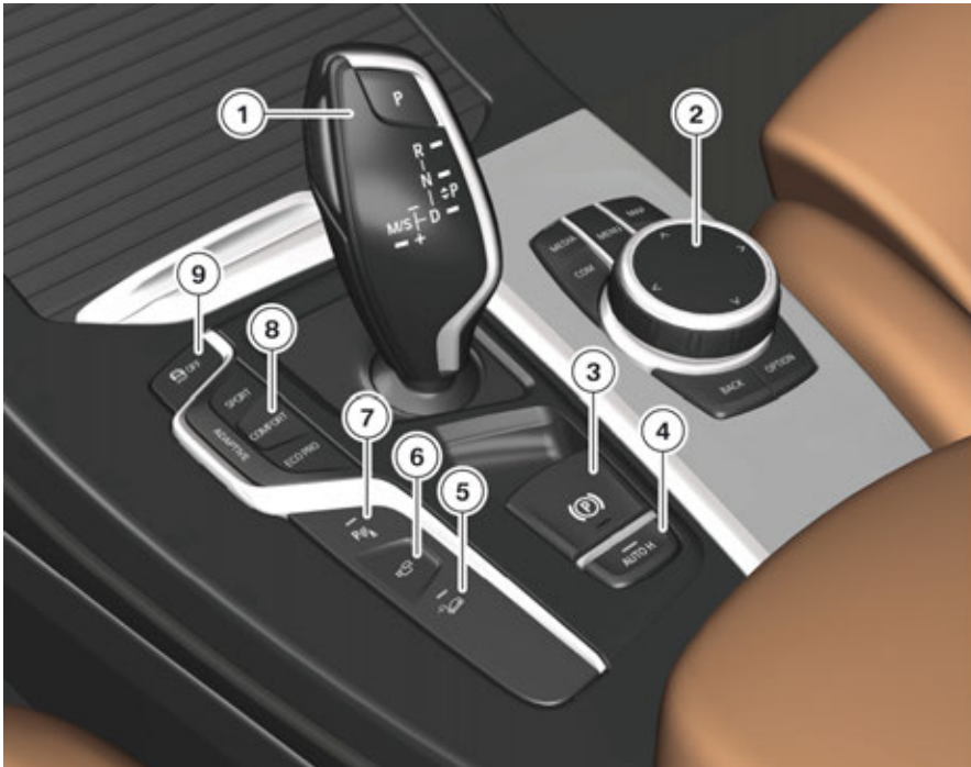
G01 Operating elements in center console
