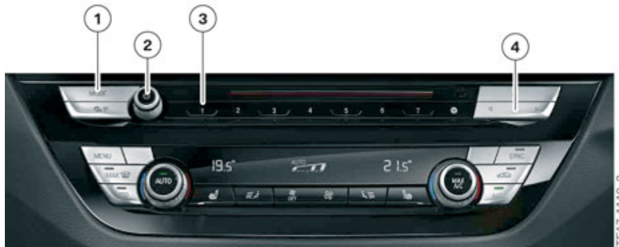
G01 Radio control panel
