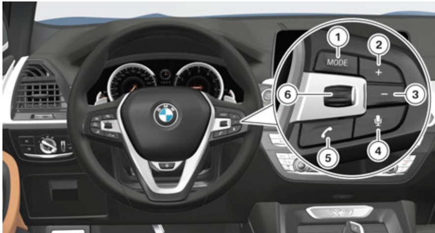
G01 multimedia buttons on multifunction steering wheel
