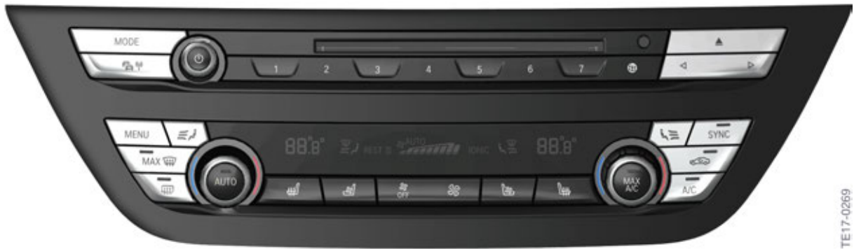
G01 3/1-zone air conditioning control panel without touch operation
